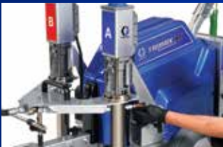
1) Remove retaining clamps and pressure transducer connections
